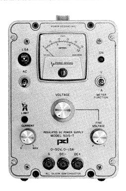
The Model 5015T is a stable DC power source designed for laboratory, industrial, and electronic-system applications. Coarse and fine controls provide continuous adjustment over the entire output voltage range. A self-indicating current limiter permits output current control from zero to the maximum supply capability. Internal circuitry completely protects the instrument from overloads and short circuits. Rear terminals are provided for external voltage programming and remote sensing.
